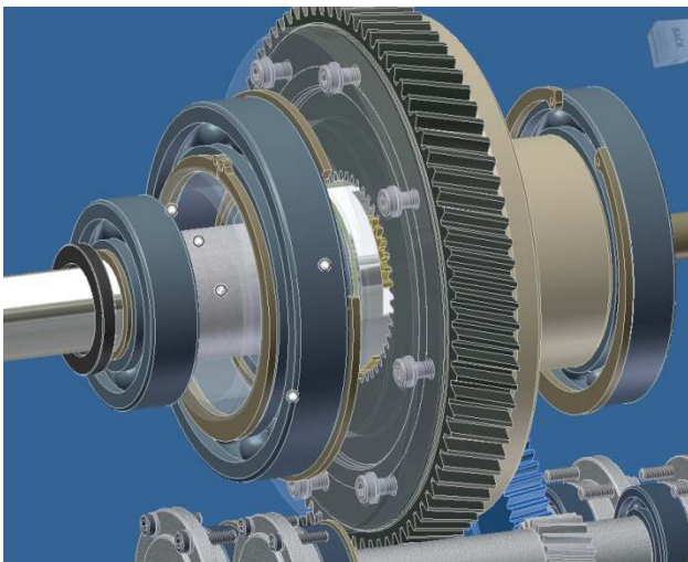
Fig. 16. Support arrangement of differential annulus gear Theoretically, if efficiency of all the prototype components
