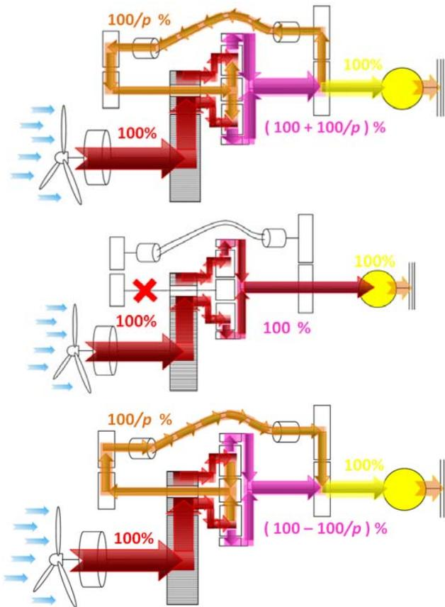
Fig. 9. Power flows in the three operating conditions
