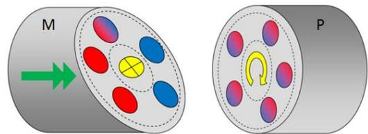
**Fig. 7.** Motor stops and pump rotates free
