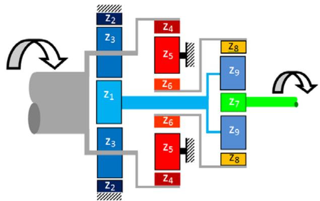
**Fig. 15.** Compound planetary transmission scheme
