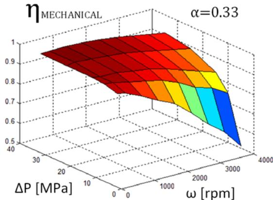
**Fig. 2.** Mechanical efficiency of the axial piston motor
