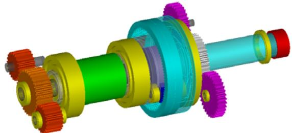
Fig. 11. Mechanical parts of the hydrostatic-mechanical transmission
