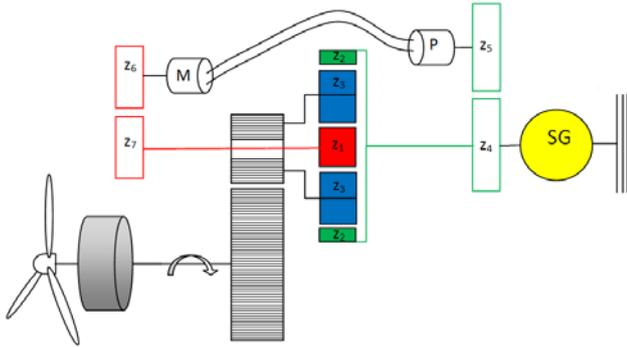
**Fig. 4.** Mechanical-hydrostatic transmission scheme
